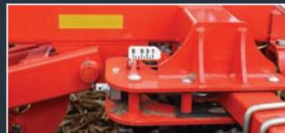
1° to 8° adjustable gang angle offers true vertical to XTended Tillage
